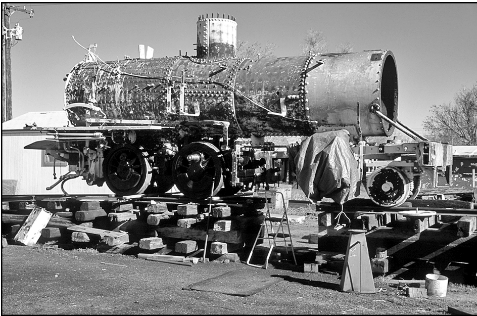
Built for the Denver, South Park & Pacific as #72 (Cooke builder number 1555) in February, 1884), Colorado Historical Society owned ex-Colorado & Southern Railway #9 was undergoing restoration for eventual operation at the Georgetown Loop Railroad. One driver wheel set was missing on 4/21/05 at the Uhrich Shop, Strasburg, CO. It was in the shop undergoing restoration work. – Photo © Chip 2005.
